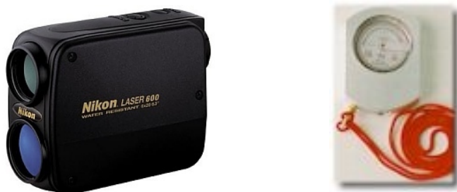
Figure 1. Left: Laser rangefinder. Right: height meter.
